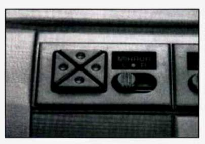
Some mirrors are manually adjustable. The optional electric mirrors come with a remote control adjustment switch. Find the switch on the instrument panel above the radio.
